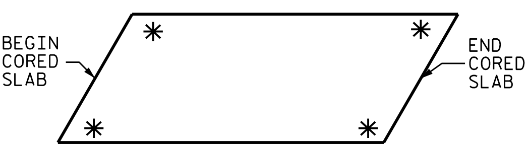
SKETCH SHOWING POINTS OF ATTACHMENT
